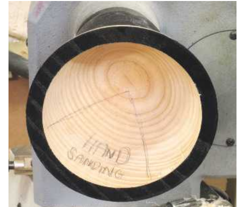
▲ Pic.6 Sanding the inside by hand or using the Pro Sander is best done in this area. I tend to power sand over at 3 o'clock as I find it easier to control the drill in that position
